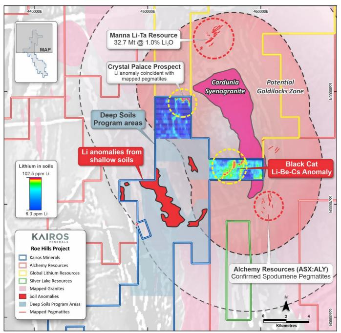
**Figure 1**. Kairos lithium anomalies at the northern half of the Roe Hills project showing the position of Manna Li-Ta deposit and Alchemy Resources' Cherry-Hickory-Pecan pegmatites. The planned deep soil sampling areas are shown in grey.
