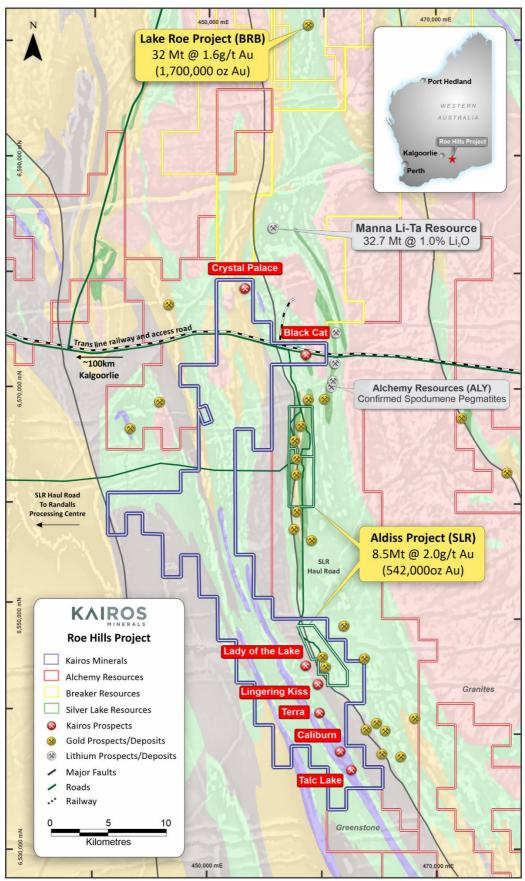
**Figure 4**. Kairos' tenements in relation to neighbouring companies over the Roe Hills area overlain on a magnetic image highlighting interpreted granites. Lithium mines and advanced projects with resources are shown with quoted resources.
