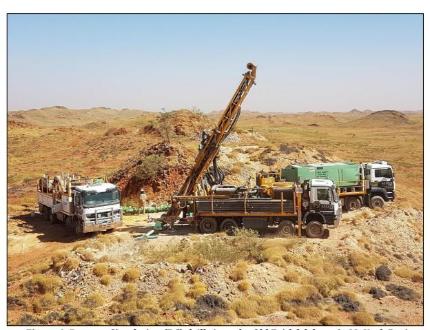
Figure 1: Reverse Circulation (RC) drill rig at the Old Faithful deposit, Mt York Project.
