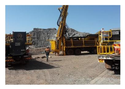
Plate 1:RC drilling at Iron Stirrup
