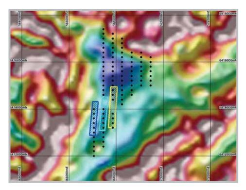
Figure 18: Fraser Range, MLEM Stations, Channel 20 (6.09 ms) and Modelled Maxwell Plate on a Total Magnetic Intensity Reduced To the Pole Image.
