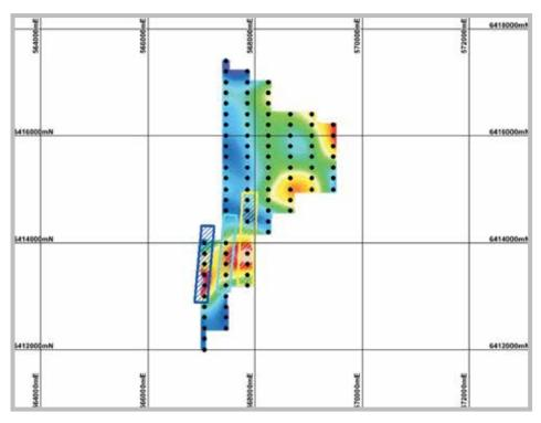
Figure 19: Fraser Range MLEM stations over MLEM channel 20 (6.09 ms) Image & Modelled Maxwell plates.
