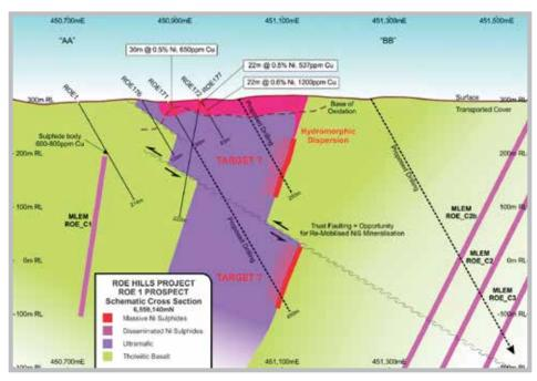
Figure 11: ROE1 Schematic Cross Section on 6,559,140mN
