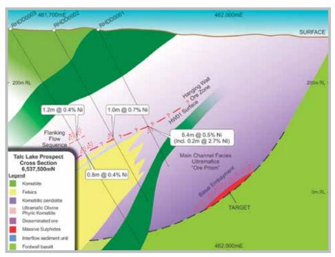
Figure 7: Talc Lake Schematic Cross Section on 6,537,500mN
