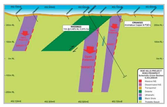
Figure 14: ROE2 Schematic Cross Section 6,553,200mN
