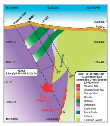
Figure 13: ROE2 Schematic Cross Section 6,553,460mN
