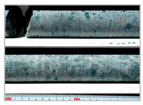
Photo 1: Core photography, TL09, depth 18-19m, Disseminated sulphide blebs in carbonated-talc ultramafics.
