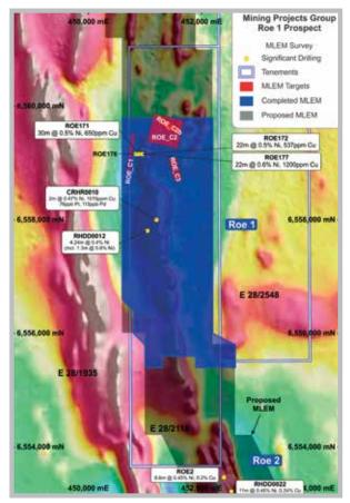
Figure 6: ROE1 MLEM Survey and Priority Conductors
