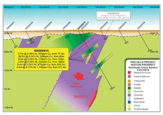
Figure 15: Hooton Schematic Cross-Section 6539,200mN.
