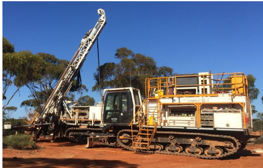
Plate1: Strike Drilling's X350 track mounted drill rig & track mounted support vehicle/booster compressor
