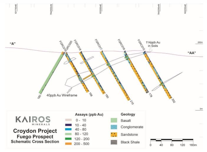
Figure 5: Drill hole section with interpretation of the mineralisation, 40ppb wireframe.
