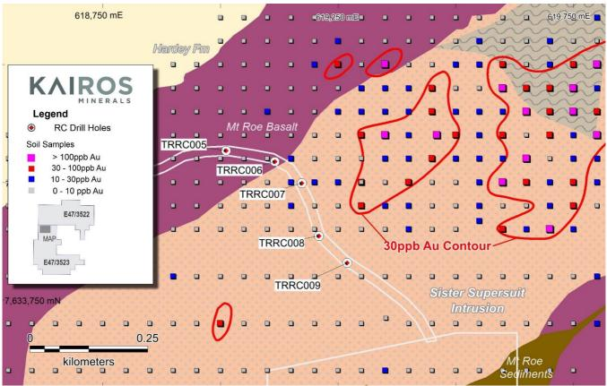
Figure 6: Tierra Prospect RC drill holes and soil anomalies over the Sisters Supersuit intrusion.
