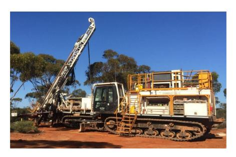
Plate1: Strike Drilling's X350 track mounted drill rig & track mounted support vehicle/booster compressor
