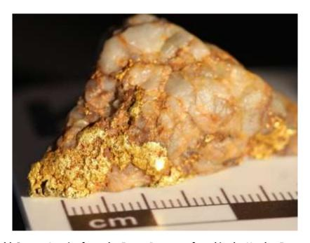
Figure 4: Primary Gold-Quartz-Arenite from the Fuego Prospect, found in the Hardey Formation sediments.
