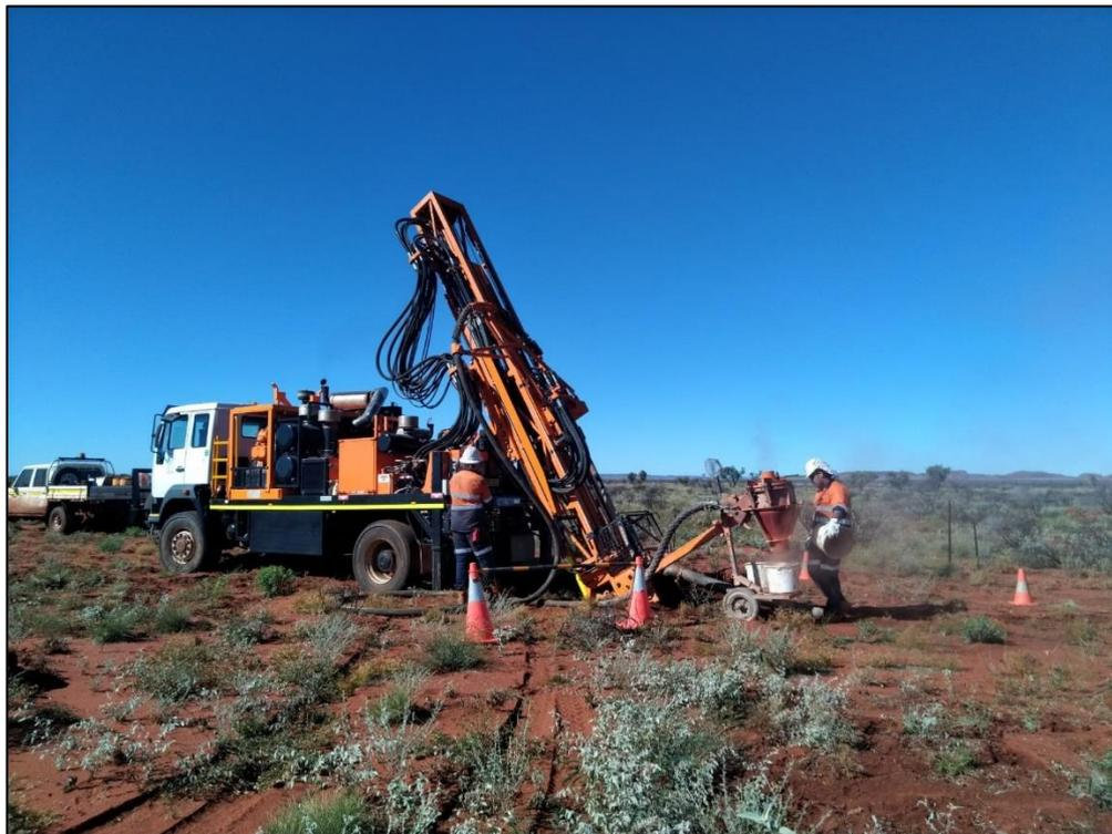
**Figure 1: Air-core rig operating at Kangan Project.**
