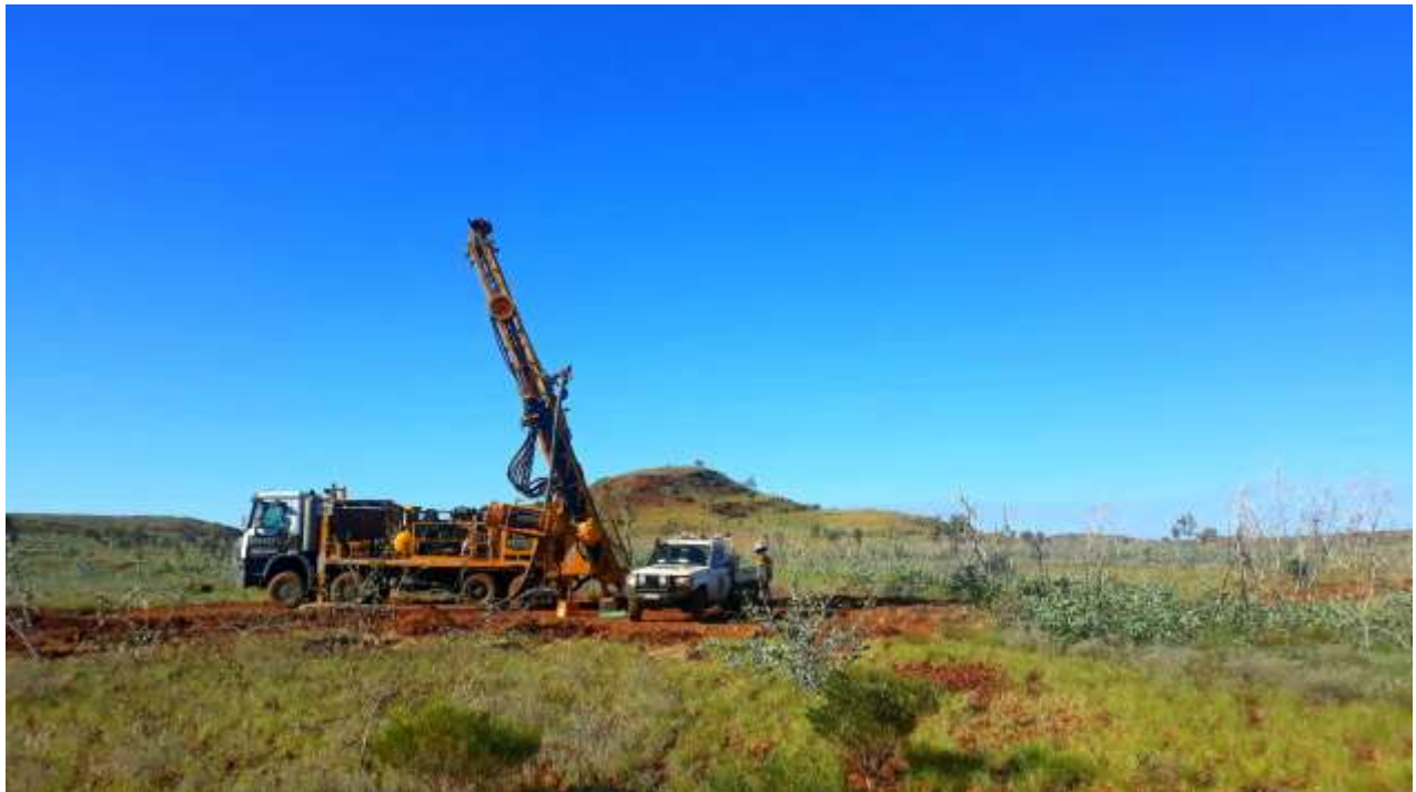
Figure 1: Mt Magnet Reverse Circulation (RC) drill rig operating at the Fuego prospect, Croydon Project.
