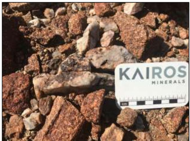
Figure 4: Photo of the quartz vein within the gabbro unit.
