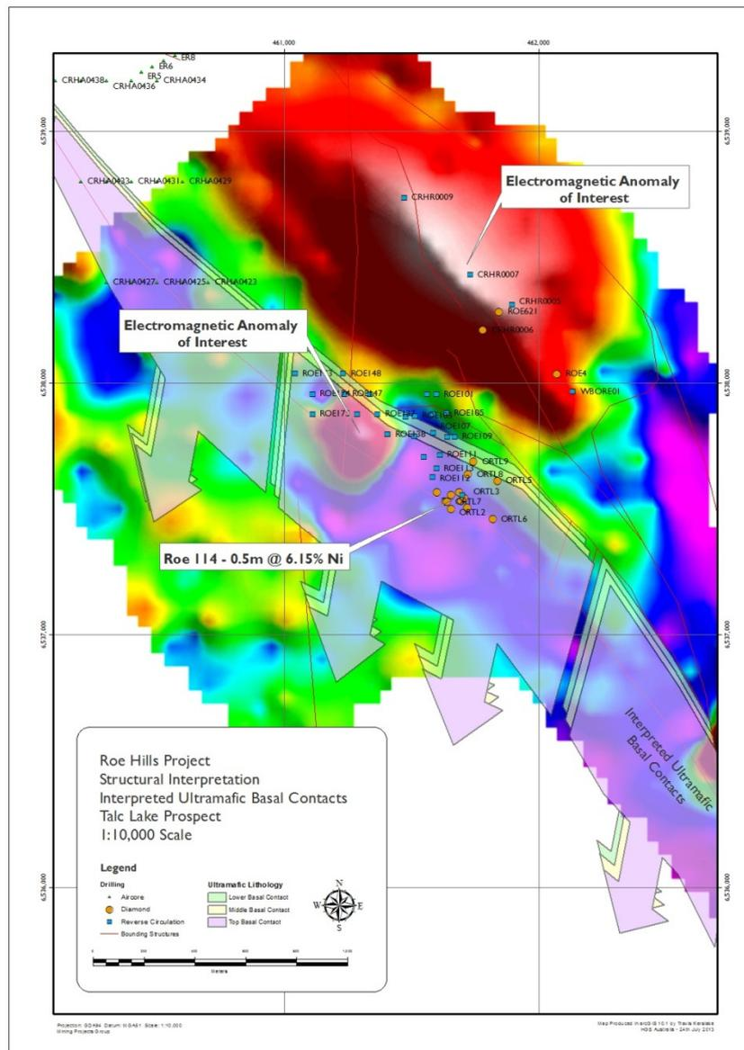
**Figure 4.** Talc Lake Prospect showing ultramafic outline and trend, and electromagnetic anomalies of interest. The translucent overlay highlights the extensive ultramafic sequence with three defined flows down dipping to the south-east which remains substantially untested.
