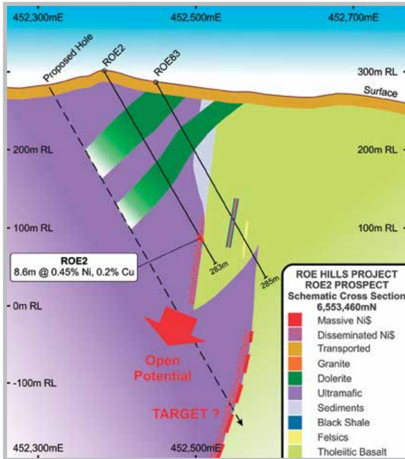
Figure 13: ROE2 Schematic Cross Section 6,553,460mN
