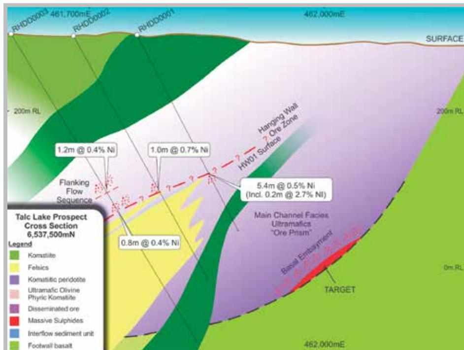
Figure 7: Talc Lake Schematic Cross Section on 6,537,500mN
