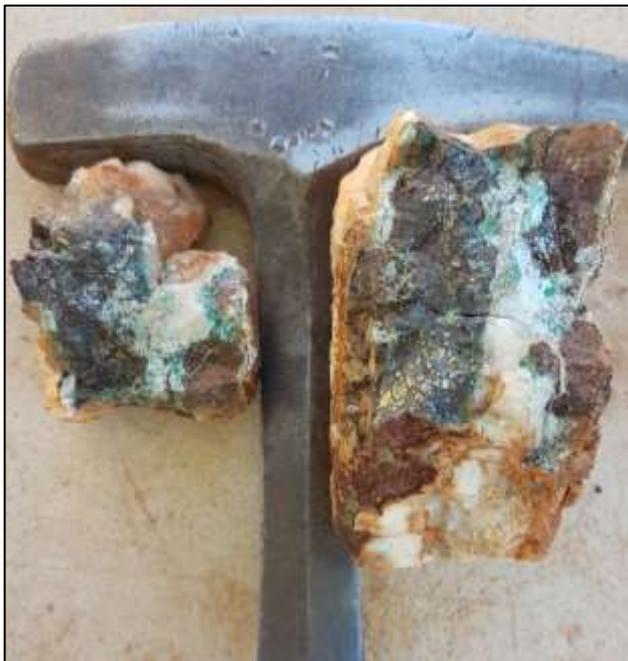
**Figure 6: Rock chips samples of the high copper-gold vein in the older Archaean basement.**
